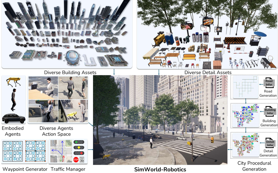
Figure 1: Overview of SimWorld Robotics (SWR). Built upon Unreal Engine 5, SWR is a simulation platform for large-scale, photorealistic, and dynamic urban environments. It offers diverse high-fidelity building and object assets, supports embodied agents with rich action spaces, includes a background traffic system powered by city-scale waypoint generation, and enables comprehensive city procedural generation.
